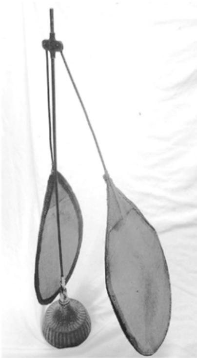
A mechanical fly-swatter. Winding up a spring set the arms in motion.
